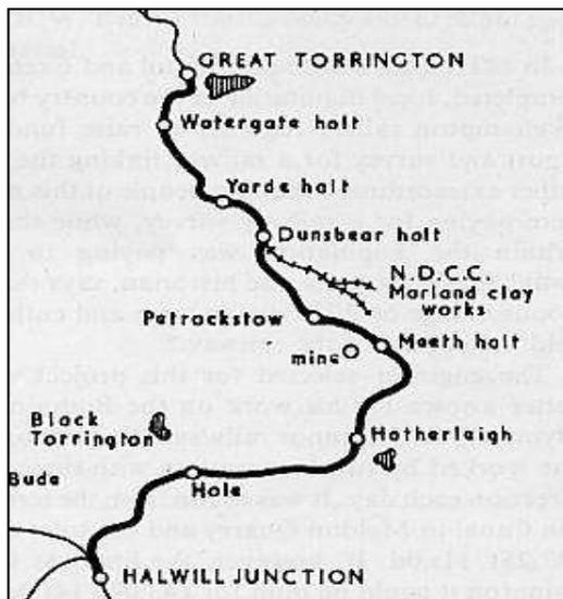
This shows the route of the 1925 upgrade to standard gauge rail by the L&SWR. The new line ran from Torrington to Halwill Junction.
