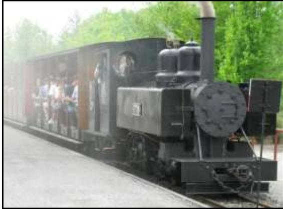
**4-6-0T Baldwin No.44656/1917** from the Leighton Buzzard Railway. One of 495 locomotives built by Baldwin for UK War Department Light Railways. They operated on the thousands of miles of narrow gauge tracks that supplied the front line trenches in the First World War. It then worked in India until the 1980s, finishing at the Upper India Sugar Mills in Uttar Pradesh.
